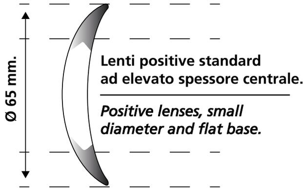
*If possible, use POSITIVE lenses, we suggest using lenses of small diameter ( $\varnothing$  50-55 mm) and flat base.*
